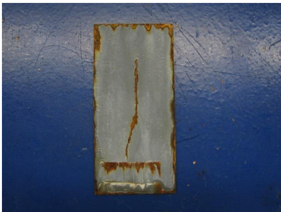
Picture 9 Zinc 720 70-90µm after 720h salt spray test
