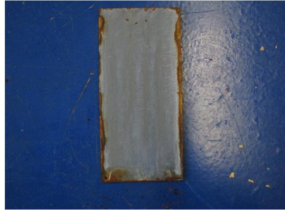
Picture 8 Zinc 720 40-50µm after 720h salt spray test
