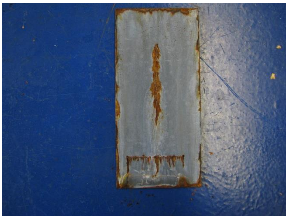
Picture 3 Zinc 240 30-50µm after 720h salt spray test
