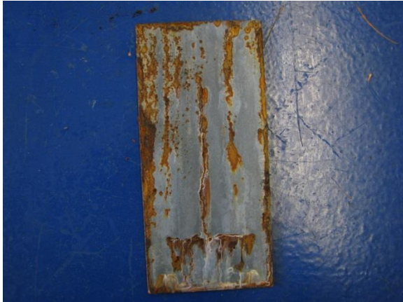
Picture 1 Zinc 240 20-30µm after 720h salt spray test
