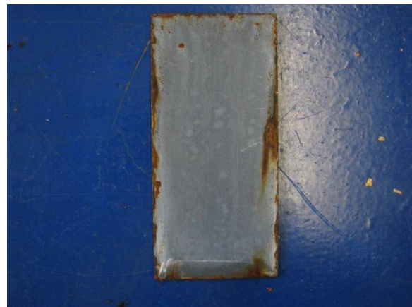
Picture 4 Zinc 240 30-50µm after 720h salt spray test
