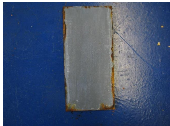
Picture 6 Zinc 240 70-90µm after 720h salt spray test
