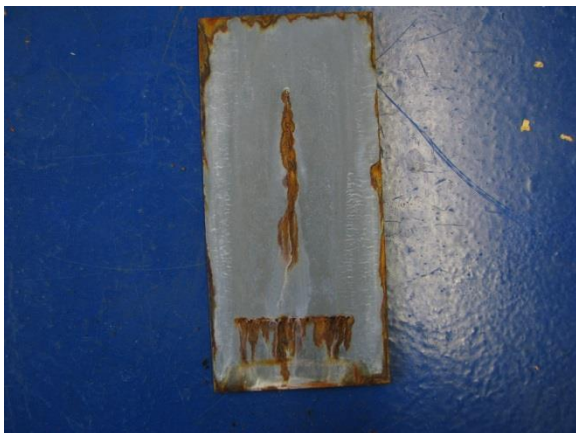
Picture 5 Zinc 240 70-90µm after 720h salt spray test
