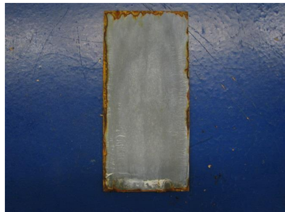
Picture 10 Zinc 720 70-90µm after 720h salt spray test
