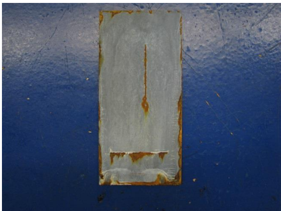
Picture 11 Zinc 720 100-130µm after 720h salt spray test
