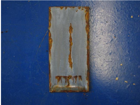
Picture 7 Zinc 720 40-50µm after 720h salt spray test
