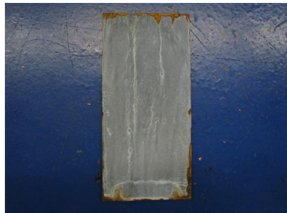
Picture 12 Zinc 720 100-130µm after 720h salt spray test
